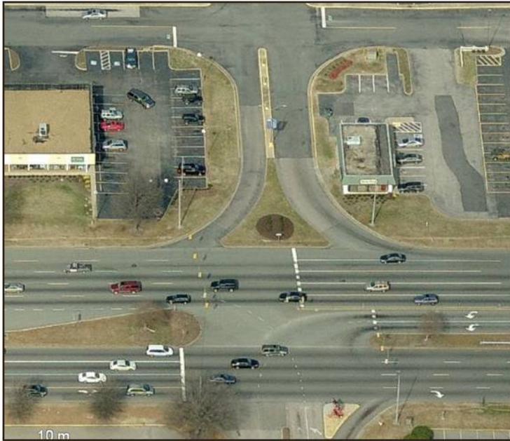
Entrance Island to Limit Left Turns
